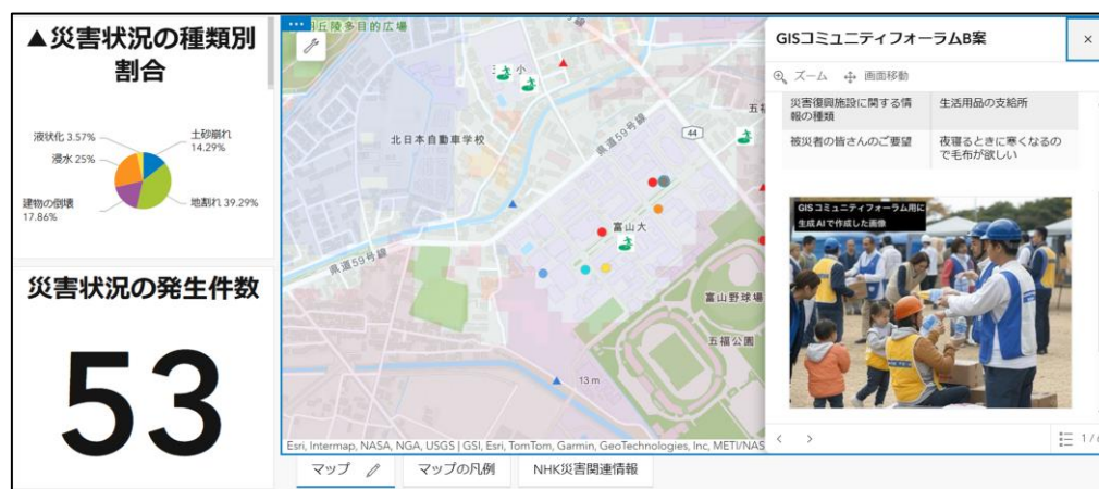
Fig. 1. Citizen-participatory disaster information sharing system using ArcGIS Online. It is a web application in which information is mapped at the center, with statistical summaries displayed on the left and individual report details presented on the right.
